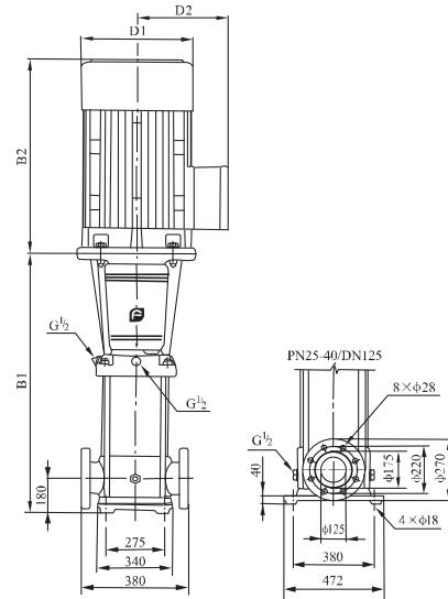
The overall dimensions of explosion-proof motor is a little different. Pls contact us for details.
