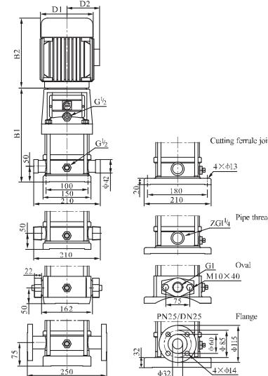
CDL1~1-36 sub-connection of pipeline has no oval flange connection.
