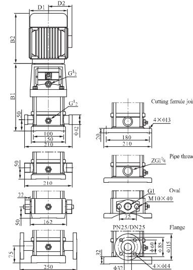
CDL3-25 ~ 36 sub-connection of pipeline has no oval flange connection.
