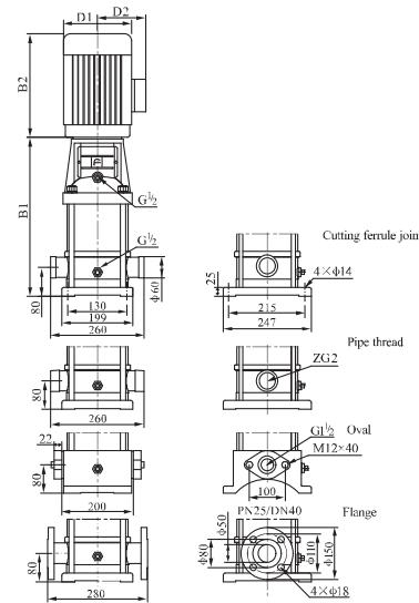
CDL8-14~20 sub-connection of pipeline has no oval flange connection.
