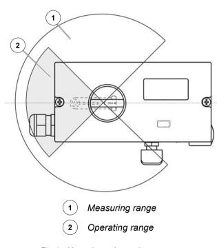
Fig. 1 – Measuring and operating ranges
