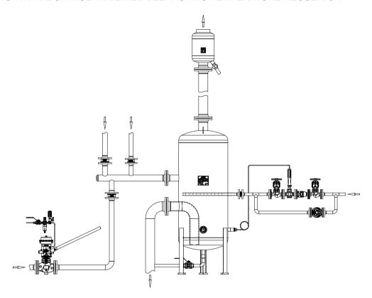
WATER COOLING AND FLASH STEAM CONDENSING WITH ADCATROL ON/OFF PNEUMATIC CONTROL VALVES
